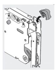
•Place the opening angle stop over the linkage pin with the arrow shaped end facing down the arm.
