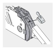
■Place the opening angle stop into the main slot and locate the 2 notches on the underside of the stop into the small cutouts.
