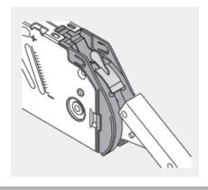
•Slide the opening angle stop in the main slot upwards away from the arm until the stop locks into position.
