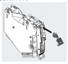
**"**Place the opening angle stop under the linkage pin with the square end facing down the arm.
