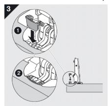
•Install stop so that the hooks lock over linkage pins
