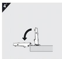
•Flip hinge arm down to opening position
