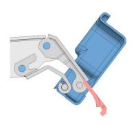
■Insert the opening angle stop into slot on the underside of hinge cup, with the tab facing toward the linkage pins.
