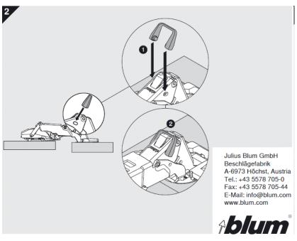
•Install stop into the oval holes below the raised Blumotion trigger point
