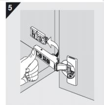
•Install hinge back onto mounting plate
