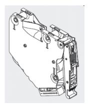
**"**Clip the hooks underneath the square end of the opening angle stop down over the plastic linkage to lock into position.
