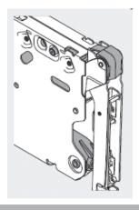
•Clip the opening angle stop down over the linkage pin to lock into position.
