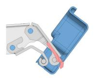
■Push the opening angle stop into the slot and ensure the tab clips over the linkage pin to lock it in position.
