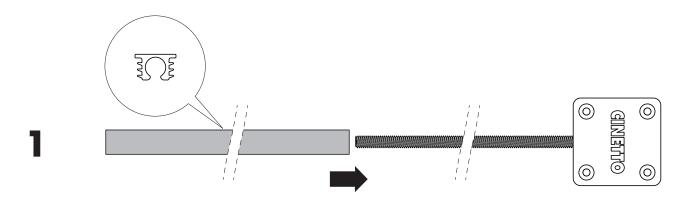
1) Slide cover over threaded rod, and push to fixed end cup
