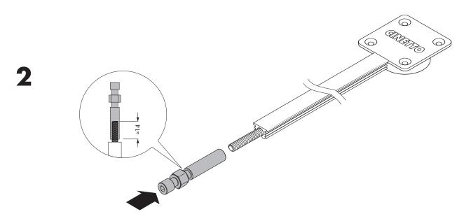
2) Screw adjustment pin onto rod, ½ way approx. 14mm. (this gives max adjustment)
